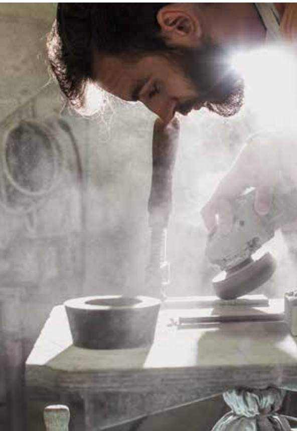
Unsafe practice: stonemason at work
